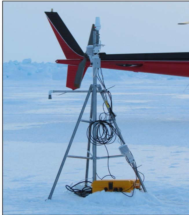
**Figure 9: CEOS IMB deployed on the mobile ice. Note the yellow logger case that houses the batteries and hardware, acoustic snow sounder deployed to the left of the tower, air temperature and pressure shields at the top of the tripod and the iridium antenna at the very top**
