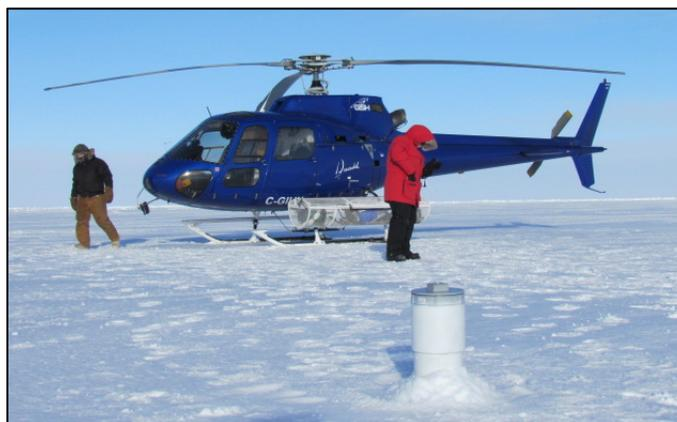
**Figure 8: Ice beacon deployed on a mobile ice floe. Approximately 12" is visible above the snow.**
