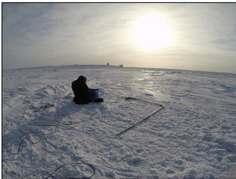
Figure 12: Preparation of under-ice light measurement through a metal arm with an attached radiometer.
