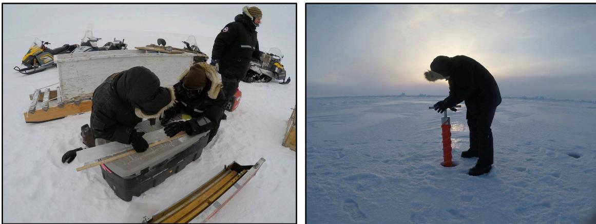
Figure 12: Left - Temperature measurements of a full ice core, Right - Sampling of bottom ice core after drilling through 70 % of the ice layer by an ice auger.
