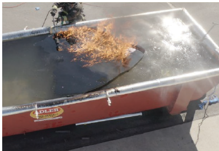
In-situ burn with simulated boom (P. Panetta & R. Byrn, Applied Research Associates)
