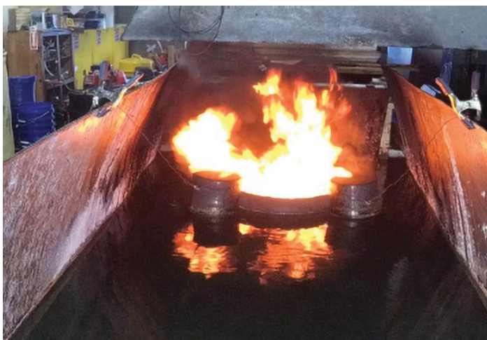
In-situ burn test of crude oil in laboratory (D. Cooper, SL Ross)
